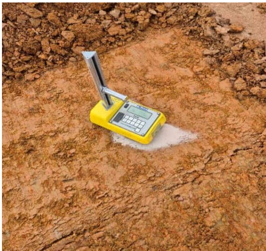
Photo 9: Field density/moisture test
