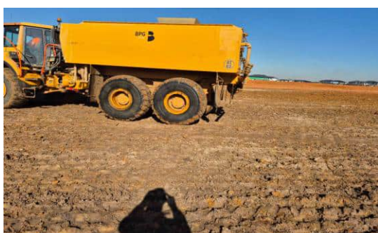
Photograph 3: Subgrade assessment with a loaded water cart.
