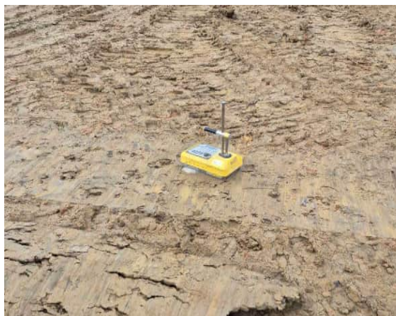
Photograph 10: Field Density / moisture test
