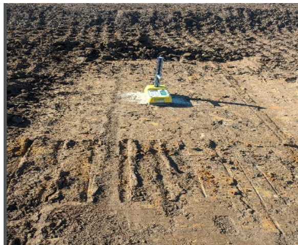
Photo 10: Field density/moisture test
