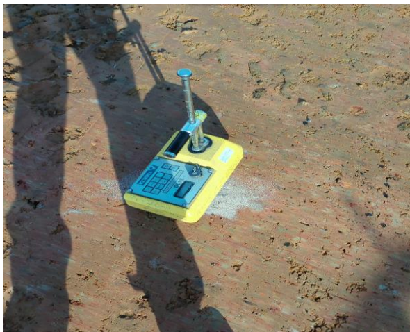
Photo 9: Field density/moisture test
